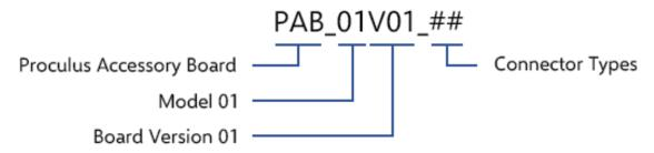
You can order PAB\_01 in any configuration of pre-assembled connector types. The following table lists part numbers for the most common (and readily available) configurations:
