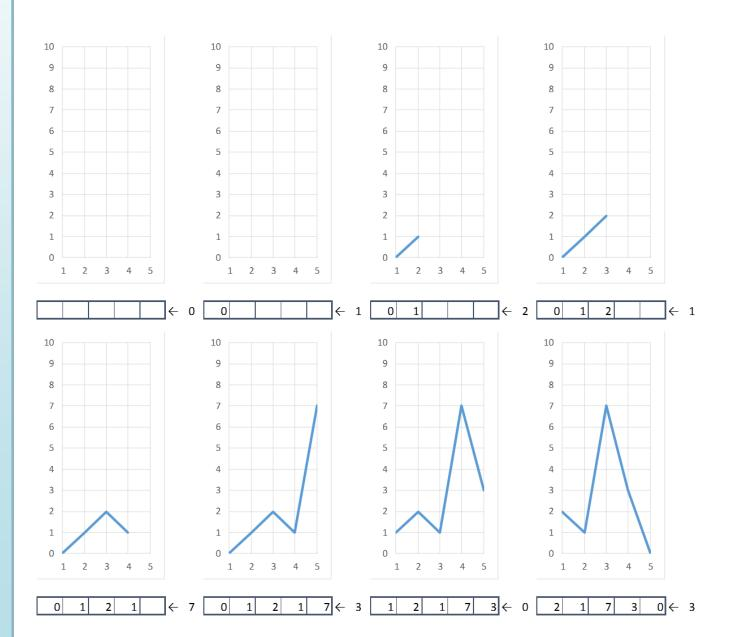
By using multiple Trend Curve Displays, you can show superimposed plots. As the curve buffers are independent from each other, the data doesn't need to be aligned.
