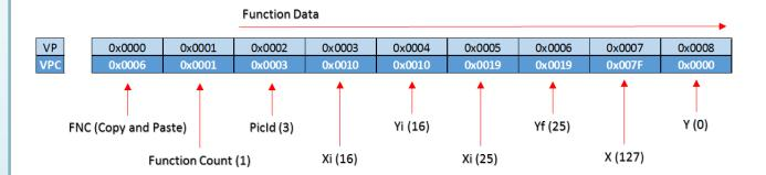
All Functions have a **Control Byte**, which is used to **finish** the displaying of graphics, or to **skip** one specific Function. To finish or skip Functions, write the corresponding value to their Control Bytes:
